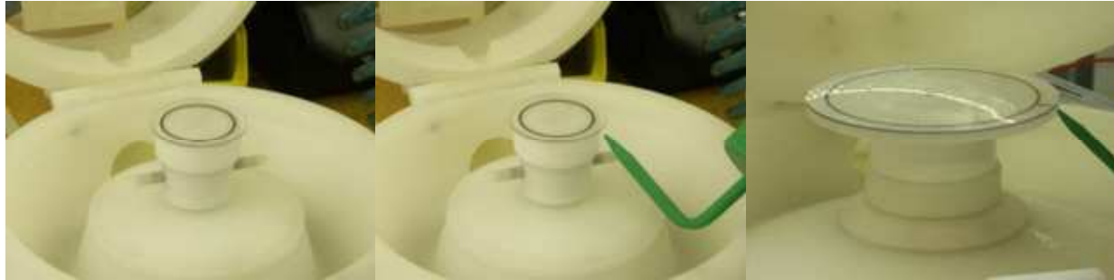
Figure 4-2 Wet Testing 1.75" and 200mm Chuck
