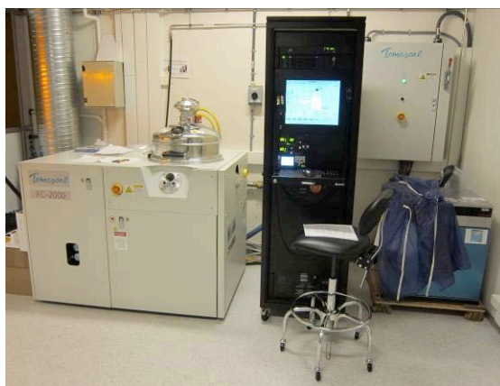
Figure 1: Temescal FC-2000 E-beam evaporator
