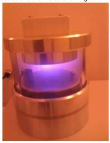
(ii) Whilst the sputtering process is in progress, outgassing of the system can alter the process current. Use the **LEAK** valve to correct these changes.
