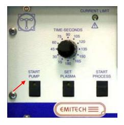
(ii) After 10-15 seconds (dependant on the size of rotary pump), the vacuum gauge will register a fall in pressure within the chamber. Continue pumping until the chamber pressure reaches 5 x 10<sup>-2</sup> mbar or better,
